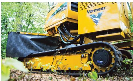
**ZERO TURNING RADIUS.** The planetary traction drive helps provide traction while the counter-rotating tracks provide tight maneuvering in difficult jobsite conditions.
