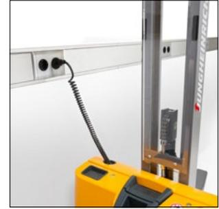
Easy charging at any 230 V mains socket thanks to built-in charger
