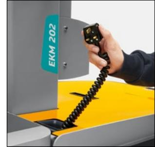
On-board charger with integrated spiral cable
